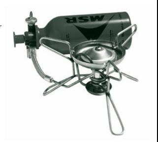
after cleaning and make sure each part is dry before reassembly. Open the valve and blow the generator out with a high pressure air hose like you find at a gas station. This clears carbon deposits which most often are the cause of improper burning. Replacement generators are available for all stoves and lanterns and will eventually need to be replaced. Please ask our staff for details if you believe replacement of your generator is necessary.
